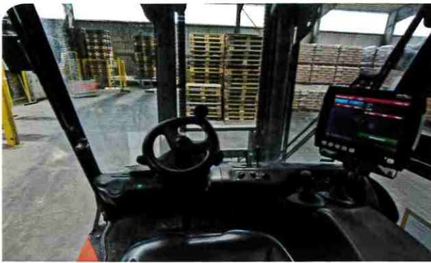
A mobile device mounted in the driver's cabin provides real-time information and allows human interactions.
